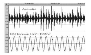
Fig.8. Acoustic emission (upper channel) during slip after application of 1000 V external periodical voltage (lower channel). Note complete phase synchronization between EM forcing and AE.
