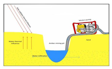
Fig. 1. Diagram of water influence on the temperature of sand dumps formed by illegal amber mining using hydraulic motor pumpsio
