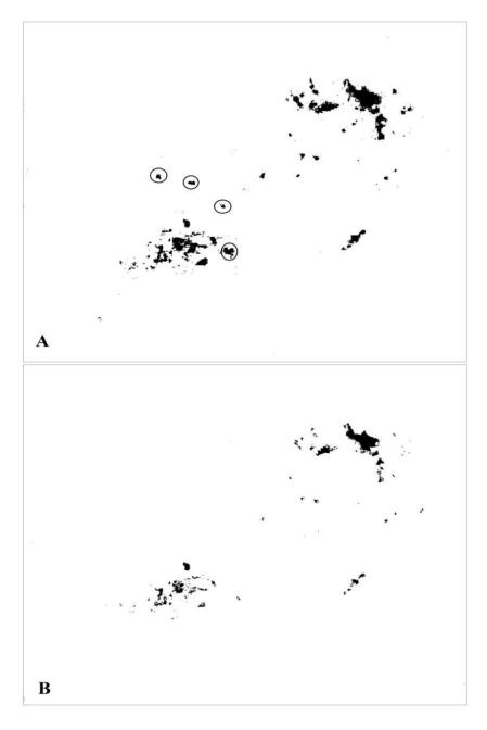
Fig. 6. Results of disturbed lands SVM-based classification. A. Based on ROI. B. Based on spectral library of sand samples. Circled areas are sand dumps formed by deforestation, first time identified on land surface temperature estimation stage.
