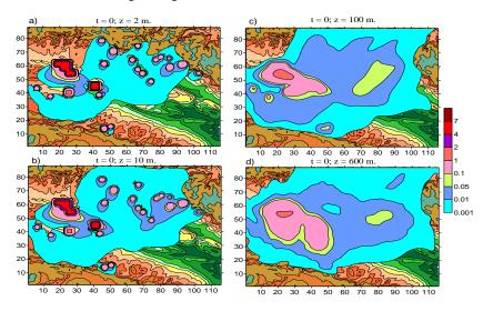
Fig. 4. Distribution of isolines of dust concentration C in MAC at a height of z = 2, 10, 100, 600 m from earth surface during background southern winds, when t = 14 hours.
