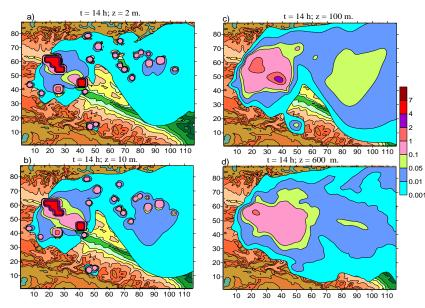
Fig. 2. Distribution of isolines of dust concentration C in MAC at a height of z = 2, 10, 100, 600 m from earth surface during background western winds, when t = 14 hours.
