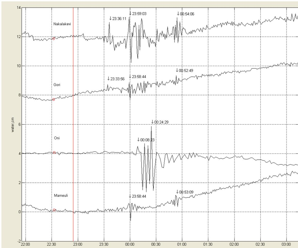
Fig. 4. WL oscillations due to passage of wave-trains of the Chile earthquake 16-09-2015,time:22:54,M8.3.Reactions successively from top to bottom in: Nakalakevi, Gori, Oni,Marneuli.
