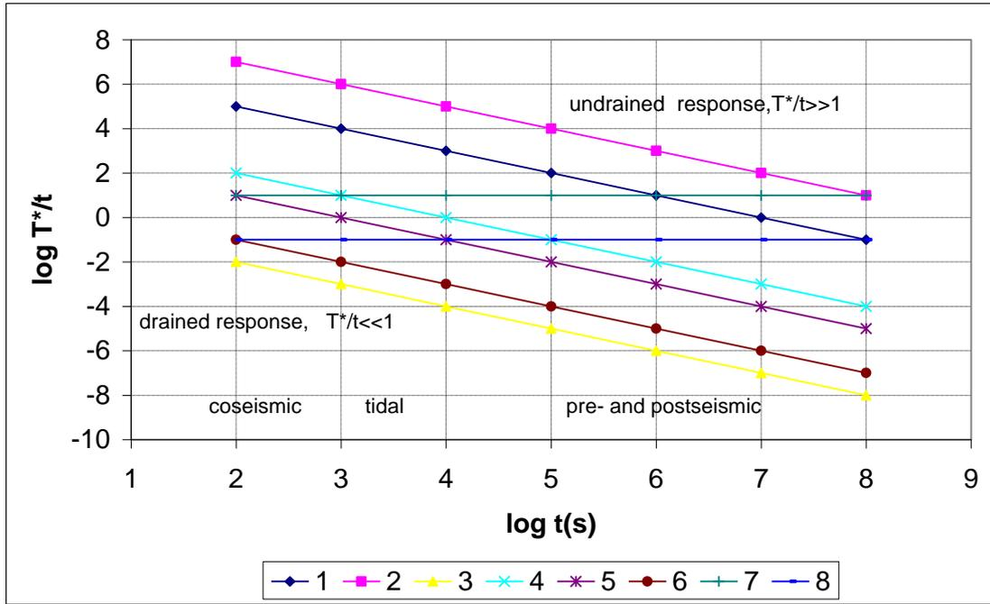
Fig.1. Hydrodynamic Fourier number  $N_{Fo} = (S_s L^2 / K) / t_e = T^* / t_e$  versus characteristic time of transient (or observation interval)  $t_e$  for various  $S_s L^2 / K$  ratios:
