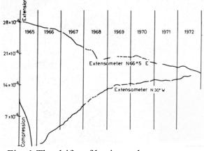
Fig. 1.The drifts of horizontal extensometer.
