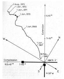
Fig. 2. The vector diagram of horizontal deformation.
