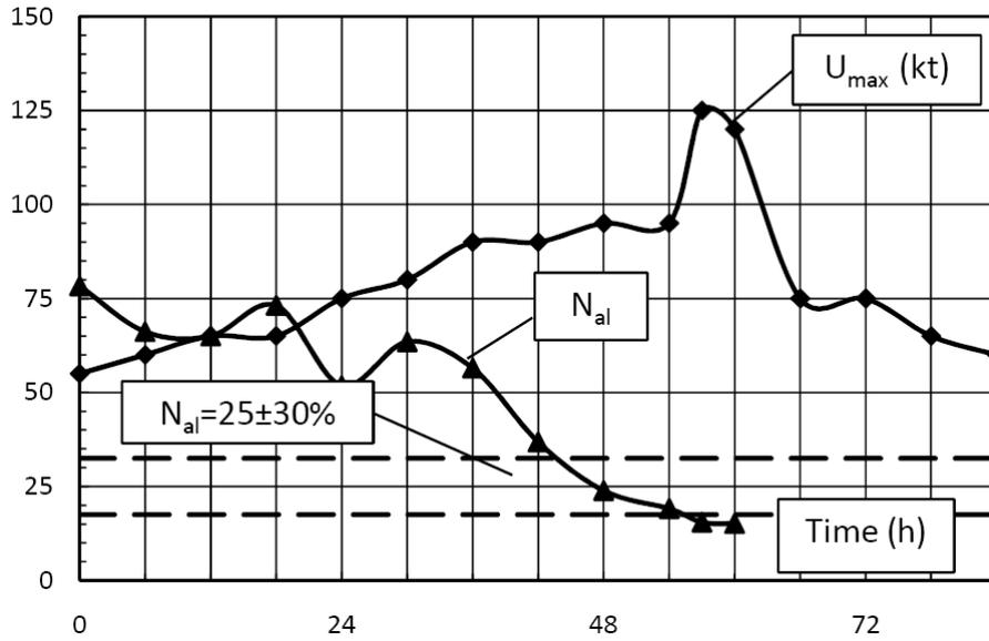
Fig. 3. Correlation of the field data on TH Charley with equation (7): the position 0 corresponds to 09:00 hour (UTC) AUG 11 2004
