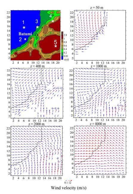
Fig. 4. The topography and wind fields at altitudes z = 50 m, 400 m, 1000 m, 2000 m, and 8000 m, respectively. Horizontal and vertical grids steps are equal 5 km.
