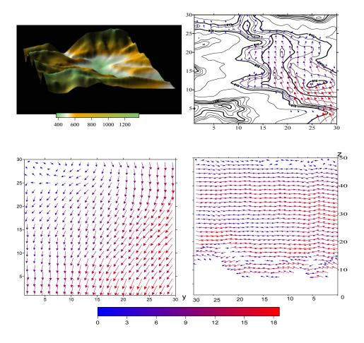
Fig. 5. The topography – (a), the wind fields at the levels z = 450m - (b), 6000m - (c) and the cross section on Y0Z surface when X = 25 in vicinity of Tbilisi city.
