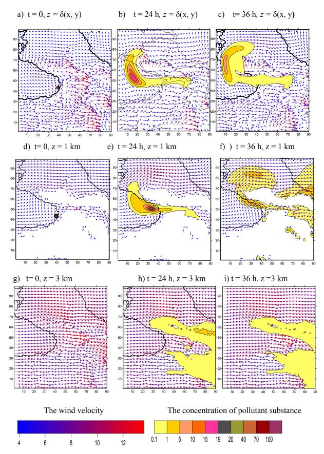
Fig. 7. The distribution of the concentration pollution substances q and the wind velocity vectors at t = 0, 24 and 36 h on the surface level of the atmosphere  $z = \delta(x,y)$ .
