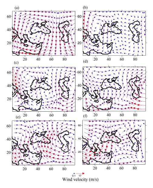
Fig. 2. The surface wind fields in the baroclyne approximation for a flat relief calculated at t = 0 h (a), 24 h (b), 48 h (c), 72 h (d), 96 h (e), and 120 h (f), respectively. Horizontal and vertical grids steps are equal 40 km.
