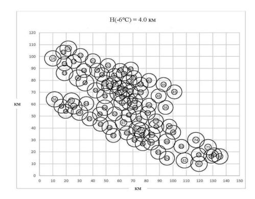
Fig. 6. Optimum areas of cloud seeding by the crystallizing reagent for the points of action by anti-hail rockets SK-6 in the protected territory in Kakheti. Height of the isotherm  $-6^{\circ}C = 4.0$  km. In the center of circle - number of the point of action.
