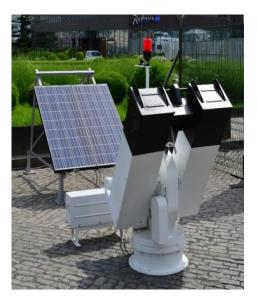
Fig. 4. The autonomous automated launching device SD-26.
