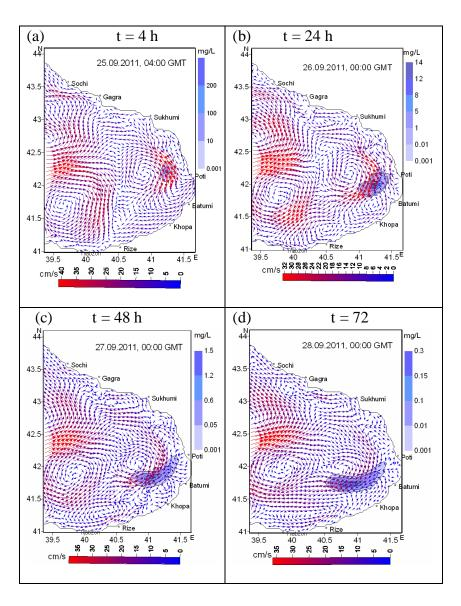
Fig.2. Simulated surface current field and oil spill transport corresponded to the following time moments after oil flood: (a) - 4h, (b) - 24 h, (c) - (48), (d) - (72). The forecasting interval is 00:00 GMT,25-28 September 2011. The source coordinates:  $142\Delta x$  and  $132\Delta y$ .
