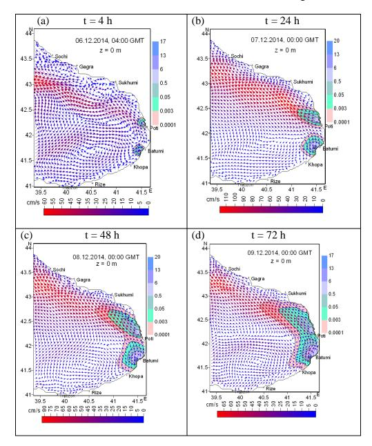
Fig. 3. Simulated surface current field and distribution of impurity at t = 4, 24, 48 and 72 h after start of getting impurity to the sea from rivers Chorokhi and Rioni. The forecasting period is 00:00 GMT, 6-9 December, 2014.
