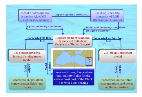
Fig.1. The forecast area, structure and scheme of functioning of the extended version of the regional forecasting system.
