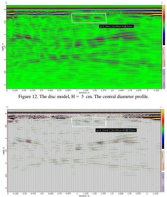
Figure 13. The disc model on the radiogram, H = 5 cm. It was constructed by placing at the depth, according to a wave image of the central diameter profile.
