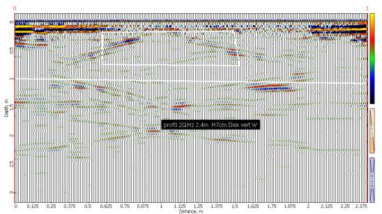
Figure 17. The disc model, H = 11 cm. Profile 3 parallel to the central diameter profile (according to the wave image).
