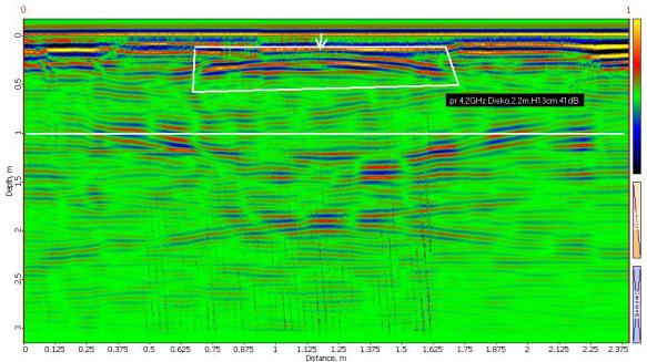
Figure 10. The disc model on the radiogram, H = 13 cm. The central diameter profile was constructed according to a density image.
