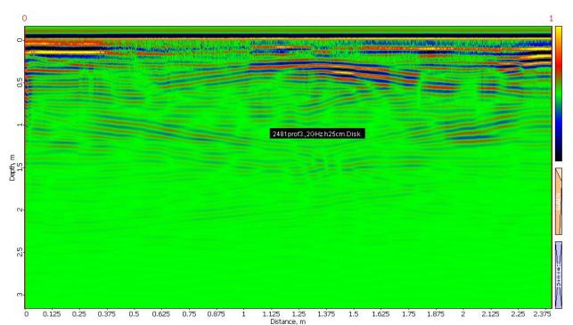
Figure 4. The disc model. The depth of the model placement surface H = 25 cm. Profile 3 passing over the disc diameter, parallel to profile 4. The distance between the parallel profiles is 0.13 cm. Profile 3 crosses the minimized part of the disc surface. 2 GHz central frequency GEORADAR antenna is used for modeling.
