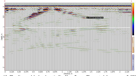
Figure 15. The disc model placed vertically, H = 7 cm. The central frequency -2 GHz. (A radiogram according to the electromagnetic wave amplitude image).
