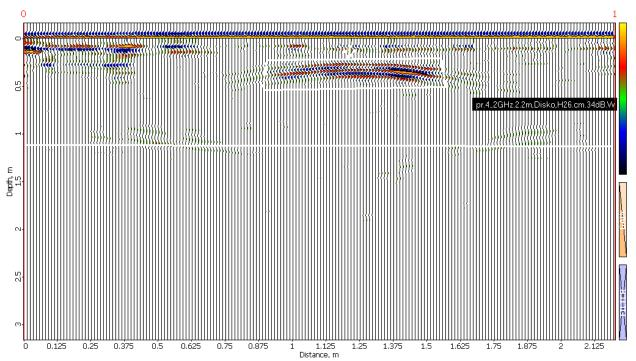
Figure 3. Central diameter profile 4 with a disc model, H = 25 cm. This radiogram shows the wave image of the profile. The maximum, minimum and zero of the amplitude correspond to the scale colours.
