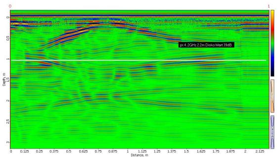
Figure 14. The disc model placed vertically, H = 7 cm. The central frequency – 2 GHz. Central profile 4.
