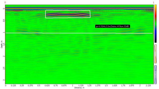
Figure 8. The disc model, H = 19 cm. The central frequency - 2 GHz. Profile 4 passing over the diameter.
