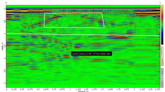
Figure 16. The disc model, H = 11 cm. Profile 3 parallel to the central diameter profile.
