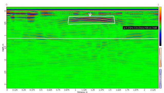
Figure 2. The model profile with void disc is given on the radiogram with wave amplitude density image. The maximum, minimum and zero values of which correspond to the colours in the scale. The depth of the model placement is H = 25 cm. Central profile 4 passing over the disc diameter. 2 GHz central frequency GEORADAR antenna is used.
