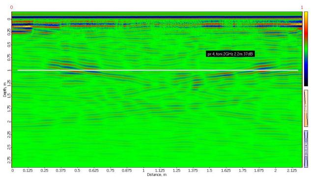
Figure 1. The background value of the field corresponding to the central profile (profile 4) of the modeling space surface without void disk. Profile length 2.2 m. 2 GHz antenna.
