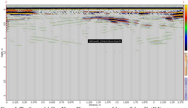
Figure 5. The disc model, H = 25 cm. The wave image of the parallel profile (No3).
