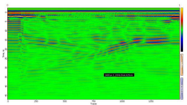
Figure 6. The disc model. The depth of the model placement surface is H = 25 cm. Profile 2 passing over the disc diameter, parallel to profile 4. The distance between the parallel profiles is 0.28 cm. Profile 2 crosses a minor part of the disc surface. 2 GHz central frequency GEORADAR antenna is used for modeling.
