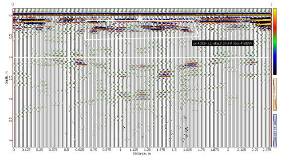
Figure 11. The disc model on the radiogram, H = 13 cm. The central diameter profile was constructed according to a wave image.
