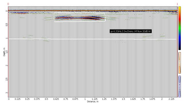
Figure 9. The disc model, H = 19 cm. The central frequency - 2 GHz. The diameter profile 4 (the profile is presented in a wave form on the radiogram).
