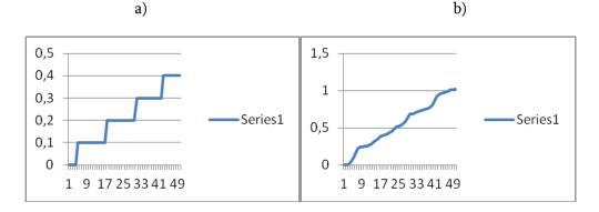
Fig. 9. a) Numerical simulation of displacement (ordinate) versus time (abscissa) for one block, b) the same calculations carried out for moving the center of gravity of the system in conditional units the Burridge-Knopoff model of four plates. (abscissa - time, ordinate - displacement).
