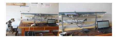
Fig.4. The Burridge-Knopoff experiments with clean surfaces plates and with a layer of sand between the plates
