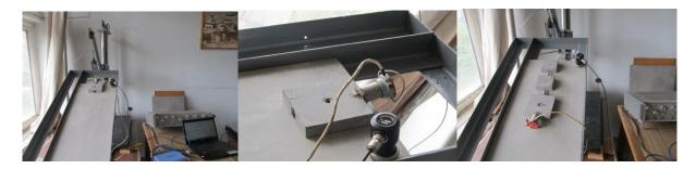
Fig. 6. Laboratory model for series of Burridge-Knopoff experiments, under the influence of gravitational forces. Middle figure shows the seismic vibrator attached to sliding plate.
