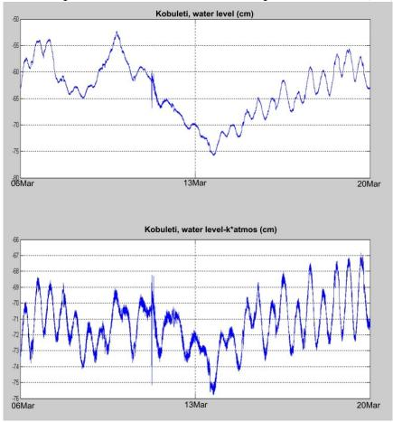
Fig. 6. WL record at Kobuleti borehole 06-20 March 2011: (a) original record of WL, absolute values, cm; (b) WL after removal of atmospheric pressure effect in reduced units; note well-marked tidal variations.
