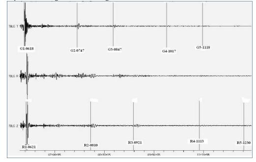
Fig.9. Seismogram with arrivals of multiple surface G and R waves at Tbilisi s/s.
