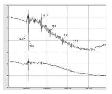
Fig.4. Water Level change in Kobuleti (top), Borjomi Park (middle) and Marneuli (bottom) boreholes before and during Japan M9 earthquake,11 March 2011 in conventional units (1/min sample rate): compressed 24 hour record.
