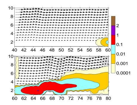
Fig. 3. Distribution of wind velocity zonal component and dust concentration C (in units of MAC) in atmospheric layer at 3 km height above Zestafoni city (y=31) in XOZ plane .
